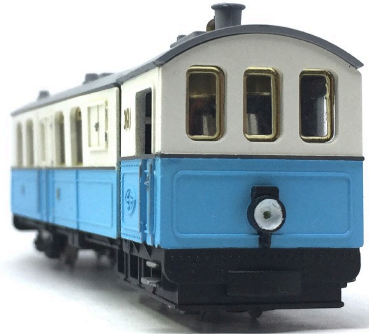
Repainted Egger-Bahn/Jouef model with Tramfabriek Coreless motor upgrade
