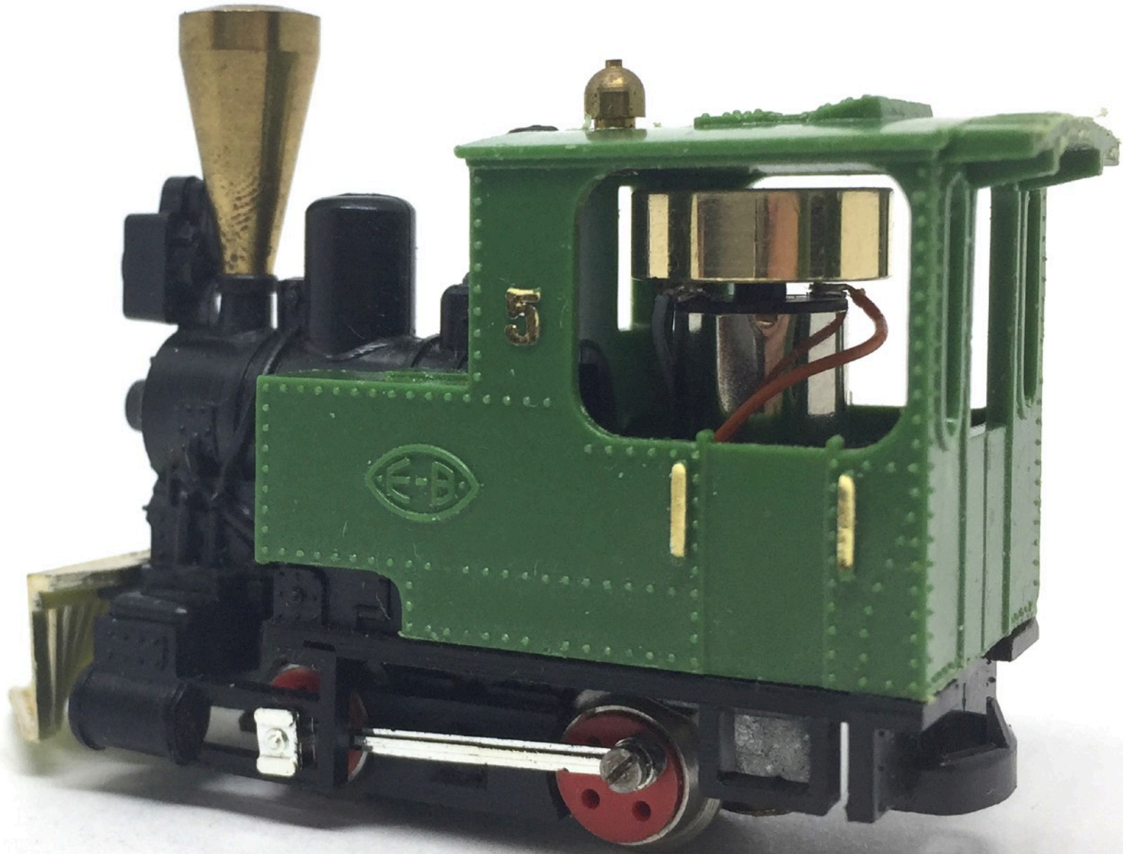
Original Egger-Bahn/Jouef model with Tramfabriek Coreless motor upgrade
