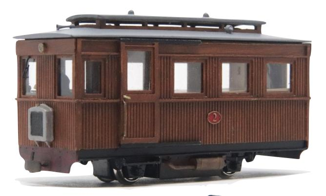
Complete brass kit with resin parts. Interior, front and rear light, motorised chassis and a (hard copy) step-by -step illustrated building instructions included.
